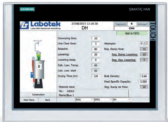
Setup menu and status for Drying Hopper
